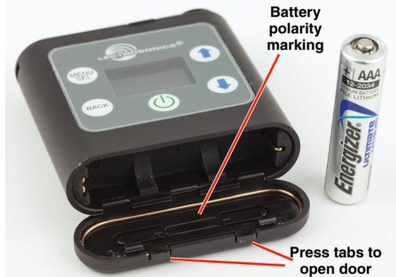
Insert the battery according to the markings inside the battery compartment door. The (+) pos. end of the battery is oriented as shown here.
